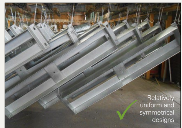
Figure 5: Avoid Distortion with Good Design
