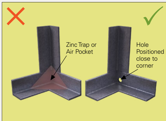
Figure 23: Inward Facing Angles – Venting Required
